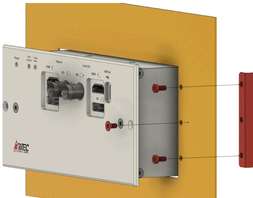
Figure 8: Etherface-1 Side Mounting example
