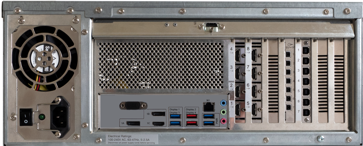
Figure 7: Rear of MDM Model EL with MDI-7, Power Breakout Board and KMS Board
