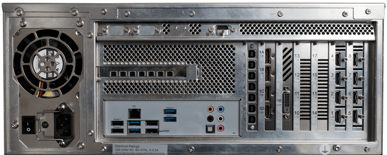
Figure 4: Rear of MDM, low-cost chassis with power supply, 1x MDI-7 input board, Power Breakout Board and KMS Board
