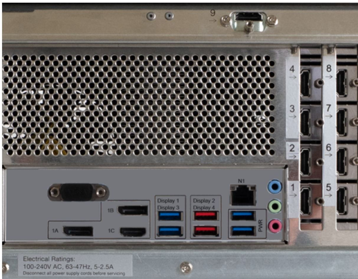
Figure 8: Detailed connector view of MDM Model EL
