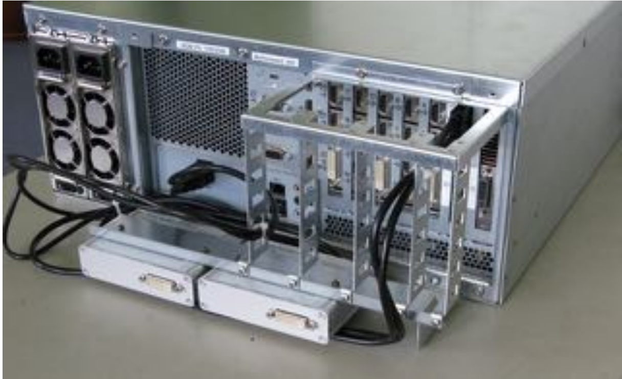
Figure 5: Rear of MDM including mounting harness
