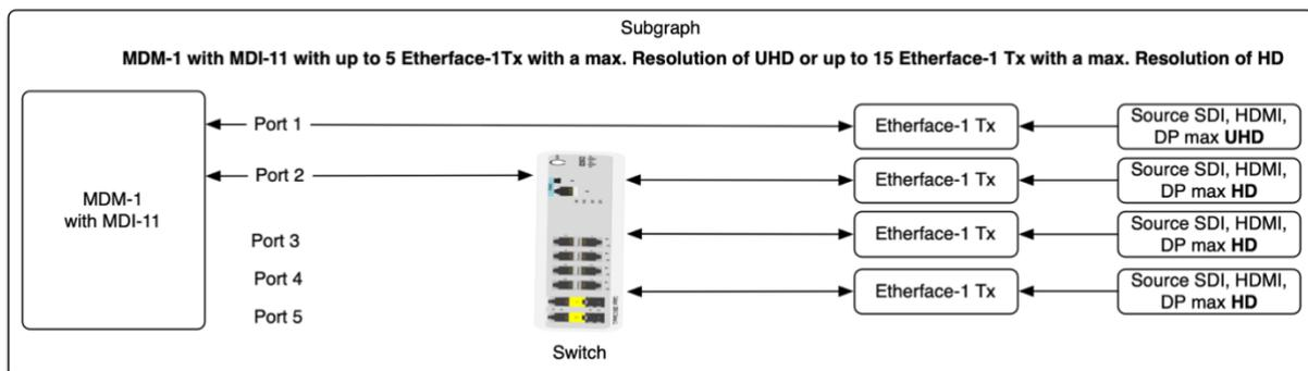
The 10G Ethernet limits the maximum resolution of the connected Etherfaces. It's the user's responsibility to obey this limitation:
