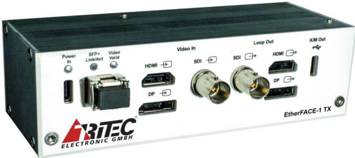
Video inputs support DP, HDMI and SDI to up to 4096x2160x60. Resolutions above UHD@30Hz will be transferred using YCbCr 4:2:2 color format. Video inputs can additionally loop-backed to local displays. USB inputs at MDM can be transferred to a PC connected at Etherface-1.
