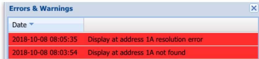
**Figure 16: Status with DP converter but no DVI connection**
