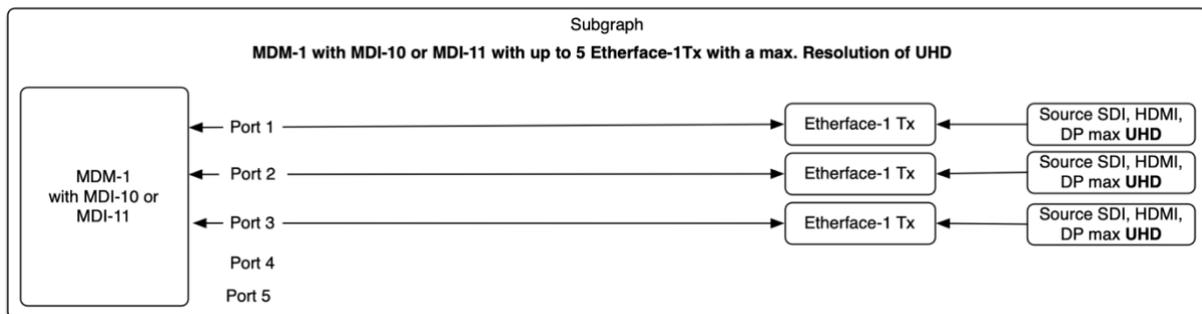
Connecting Etherface-1 Tx is plug and play. A name can optionally be given to each Etherface-1 Tx to identify it on-screen when connected.
